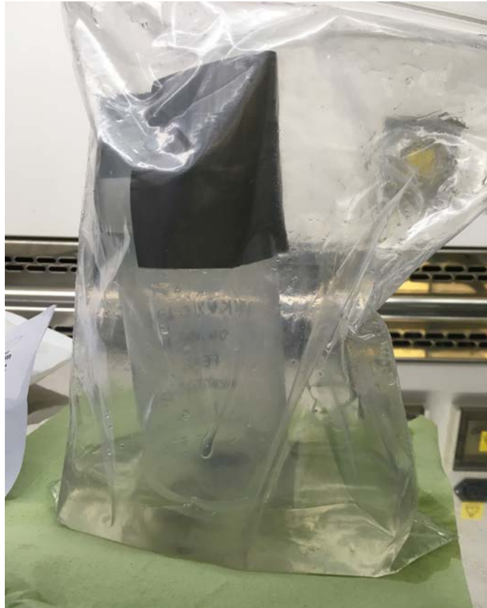
Figure 53. An example of bad packaging – no absorptive material was used. The formalin leaked out of the primary container, through the plastic bag and was leaking through the postal envelope. The primary container and amount of formalin was also excessive for the two small samples submitted
